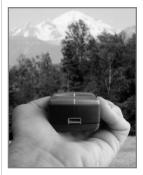
When using the 'Sight 'N Go' or 'Set Course' feature of the eTrex Summit, hold the unit level and align the Sighting Marks on the case with a distant landmark.
