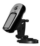
While mounted in a car or on a bicycle the eTrex Summit will be tilted enough for the Electronic Compass to become inaccurate. The eTrex Summit will automatically switch to a GPS heading when you exceed 10 mph. To switch back to the compass press and hold the **PAGE** key or wait 90 seconds after slowing below 10 mph.
