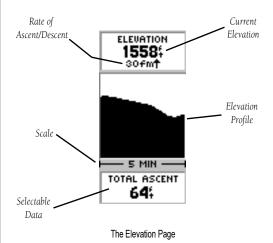
The Elevation Page will provide the user with the current elevation, rate of ascent/descent, and a profile of elevation changes over distance or time. The UP or DOWN button can be used to scroll through a variety of user selectable data including Local Pressure, Max Descent, Max Ascent, Avg Descent, Avg Ascent, Total Descent, Total Ascent, Min Elevation, Max Elevation, 12 Hour Pressure Trend.
