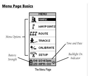
The Menu Page gives you access to e Trex Summit's more advanced features. With the Menu Page you can create and view waypoints, create a route, save and view track logs, calibrate the electronic compass and altimeter or access the system setup features. Information on each of these advanced features is included in the Reference Section of this manual.
